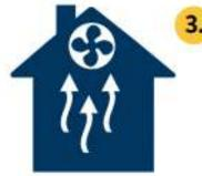
Vacuum Effect – Appliances (water heaters, fireplaces, clothes dryers, older furnaces, etc.) and exhaust fans remove air from the home. This can drive soil gas into the home as make-up air enters from the lower part of the house.
