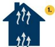
Stack Effect – Warm air rises to the upper part of the home and is lost to the outside air. Make-up air enters the lower part of the home. Some of that make-up air comes from the soil.
